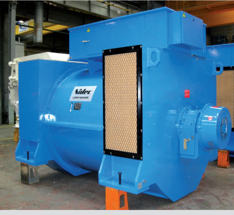
LSA 58 alternator destined for use in a power station equipped with filters
